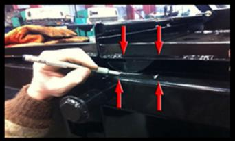
Once lid is aligned, mark the length of the hole to be cut for locking tab to drop into, being sure to use the tab as a guide.
