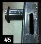
To cut locking tab slot, first drill 2 pilot holes (#1) and then use a 1/2" bit to finish the holes. (#2) After drilling, (#3) use a cordless cutoff wheel (#4) to cut out the remaining material leaving a 1/2" wide slot (#5) for the locking tab to enter the bin channel. Fold lid back over and check for clearance. If needed trim additional material from slot to make sure tab slides easily in when closing lid.
