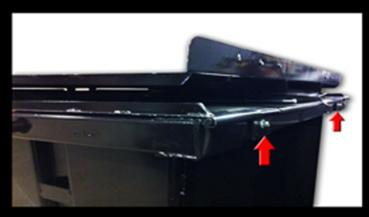
Begin by centering lid on bin with hinge plates to the back of the bin. Drill 2 1/2" holes and use a 3/8" bolt to secure lid.
