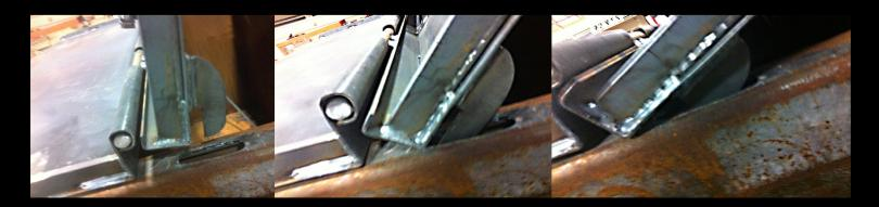
When folding lid over after cutting locking tab slots, be suer there is enough clearance for the lid to easily fold over and that the locking tabs do not catch on the edge of the bin channel. Once it is determined that there are no issues with tab clearance, the lid is ready to be locked.
