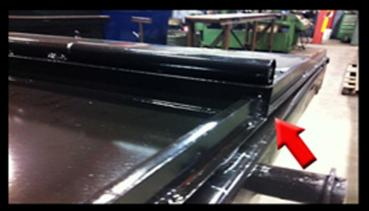
After securing lid, unfold and use a straight edge to ensure the front and rear sections of the lid are lined up for proper slot cutting placement.
